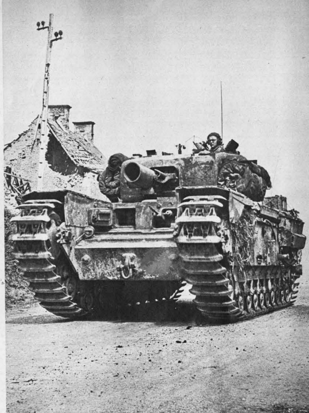
BIG MORTAR IN CHURCHILL TURRET IS CALLED THE "PETARD"; ITS PROJECTILE, "DUSTBIN"
